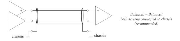
On some older items of equipment the screen connection may still be referenced to the circuit 0V rather than the chassis. In these cases it may be advantageous to disconnect the screen at this connection. Note however that this practice will degrade the EMC performance.
